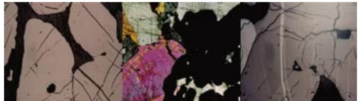
Photomicrographs of titanium ore (from left to right): 1) subround ilmenite (reflected light); 2) plagioclase, olivine and titanium oxides (polarized light); and 3) magnetite with ilmenite lamellae and ilmenite (reflected light).
