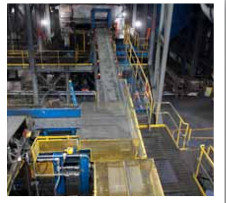
Conveyor belts move green pellets to the oven for drying.
