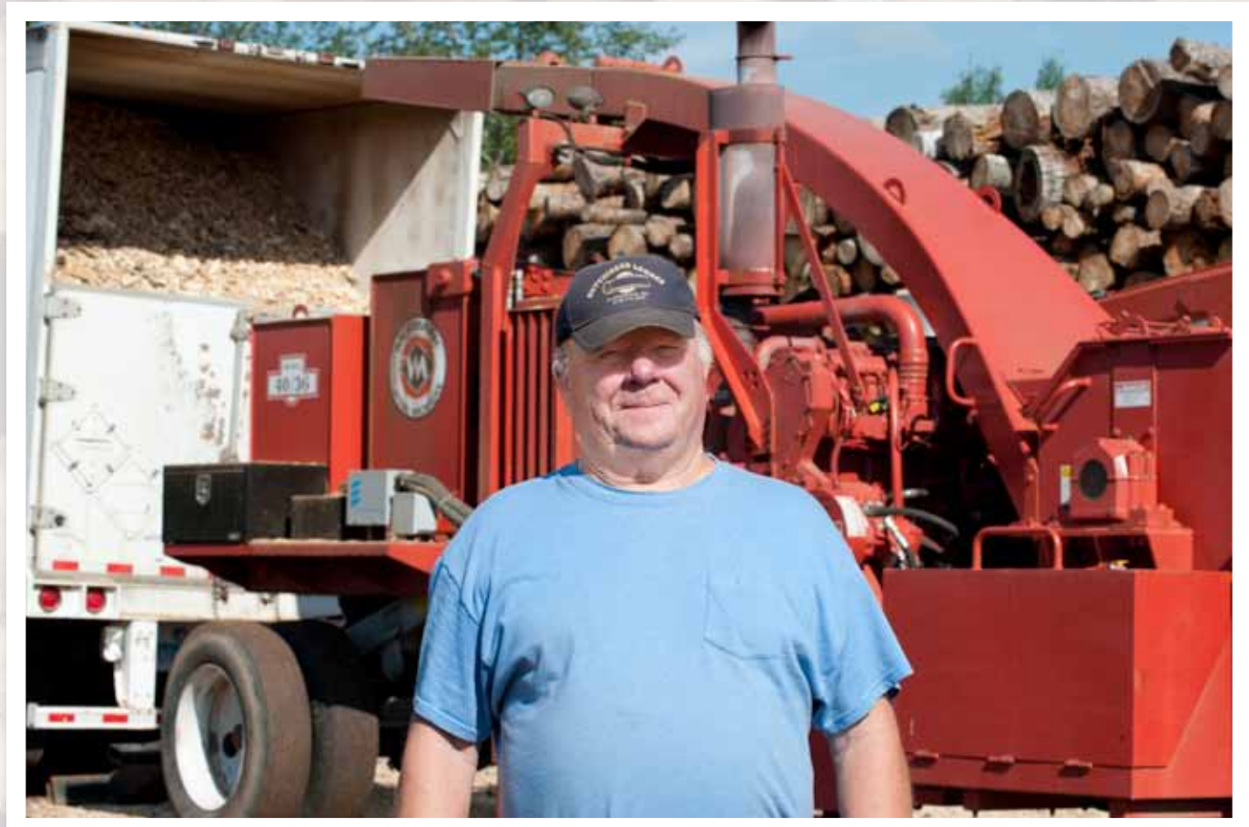
"Red" Haley, 2nd generation logger/owner of Haley Logging Company, shows off the new wood chipper used to convert logs up to 24" into wafer sized biomass.
